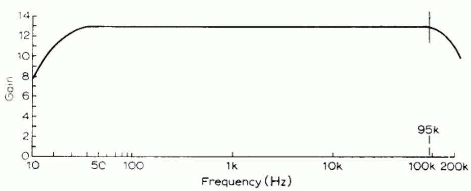
**Fig. 4. Gain/frequency response curve of amplifier.**
