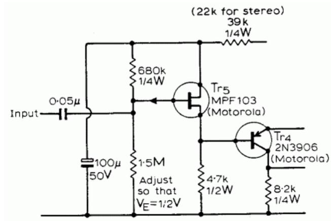
Fig. 8. Modified input circuit for high input impedance.
